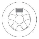
If **OPPOSITE WEIGHT FUNCTION** is enabled, the eventual application position for the bottom weight (6 o'clock) is also indicated next to the positioning arrows to facilitate cleaning the rim and the relative application of adhesive weights. The symbol used is:
