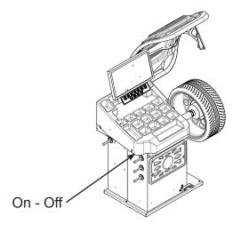
7. Position the wheel on the terminal with the inner part facing the balancer;
