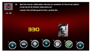
Measure the distance between the reference line on the sonar protection and the plane of the calibration device opposite to the sonar
