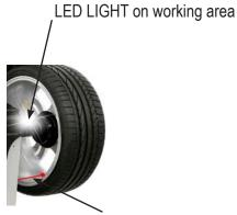
LASER LINE for exact positioning of adhesive weights.
