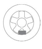
Just before reaching the weight correction position, the LED light comes on. When reaching the exact weight correction position, the LASER activates.
