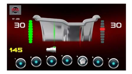
Pull out the gauge until the counterweight applicator reaches the previously selected area, FI or FE.
