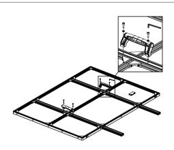
**Step 1**: Align the screw holes on two handles with those on the back of the pattern board. Place the flat washers (M5) over the screw holes and then insert bolts (M5x16) and tighten using the hex L-wrench (4mm).
