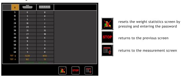
Each horizontal line indicates the number of clip-on and adhesive weights used to balance the wheels in the period between the two dates indicated on the screen (in square brackets).
