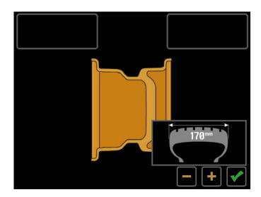
Set the width value shown on the tyre and proceed with balancing the wheel.
