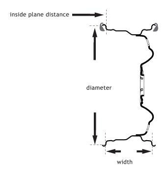
• Standard dynamic balancing using adhesive weights or a mix of adhesive and clip-on weights:
