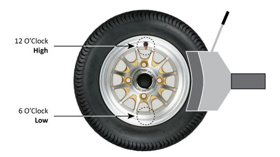
7. Move the Blade so that it is on the side of the Tire, very close to, **but not touching**, the Rim.
