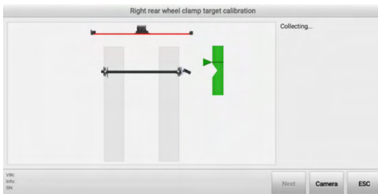
Figure 4-31 Start Calibration (Use Calibration Bar) 3
