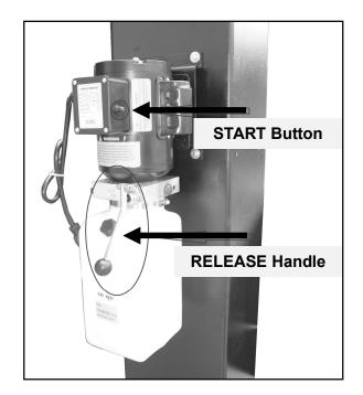
Fig. 14 Start Button & Release Handle on Power Unit
