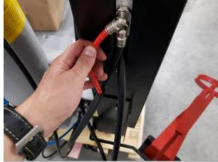
21.Manually separate the fitting from the valve so it can be installed more easily on the vertical post. ADD TEFLON TO THE FITTING OF THE VALVE (BEAD SEATER)
