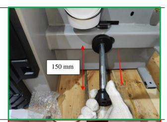
13.Remove the nut (changed the picture with the one having the rod pulled out at the most convenient distance)
