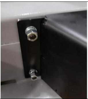
SECURE THE TOWER WITH NUT AND WASHERS TO THE BACK PLATE
