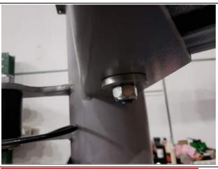
7 . REMOVE THE SCREW ON TOP OF THE ARM (OR THE ONE ON TOP OF THE LOCKING BRACKET) (*The most updated version use different screws*, )
