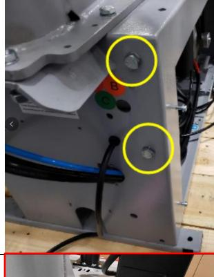
18. Fix the TOO TRAY to the body with the 2 bolts previously removed (the support of the gun has changed)
