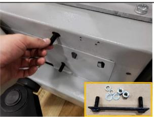
SCREW THE LONG FOOT/KNOB INTO THE BOTTOM PART OF THE ASSIST ARM TOWER
