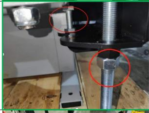
46. The disc arm and the black roller auxiliary arm are respectively placed at the bottom and top of the tower (inserted a new picture without the old wheel lift and put the 2 steps regarding the installation of the arm on the same picture)
