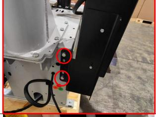
19.CONNECT THE BLACK HOSE TO THE BOTTOM FITTING (BEHIND THE ACCESSORY RACK)
