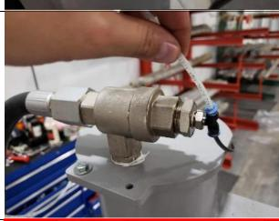
28.Take out the black hose from the tire changer body and the insert it up to the small iron pipe welded on the vertical arm. (in the new version there is not blue hose)
