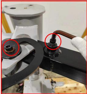
8 . PLACE THE ARM BETWEEN THE LOCKING BRACKET AND REMOUNT THE SCREW (new version use a different screw)
