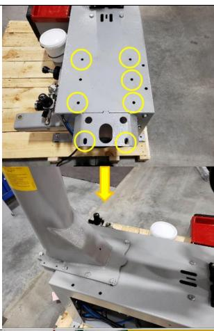
5. SET THE SWING ARM IN POSITION AND PLACE THE 2 SHIMS, BETWEEN THE ARM AND THE TOWER
