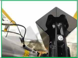
50.Place the protective cover in place and secure the screws
