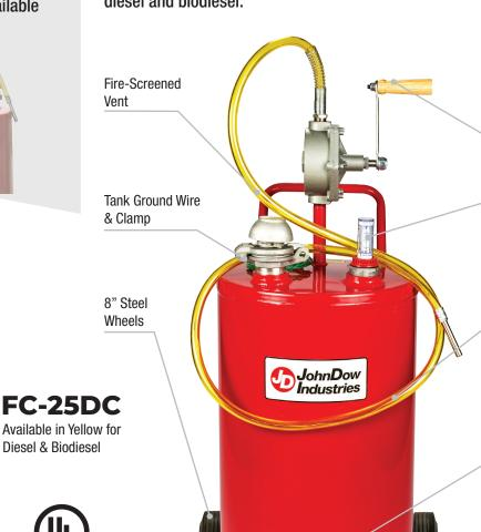
**UL Listed Cast Iron Rotary** Pump With Carbon Vanes & Viton Seals. Siphon or Dispense Fuel. Every 12 Revolutions Delivers One Gallon.
