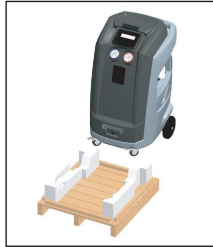
Fig. 12: Lowering unit from the pallet
