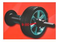
Affix the calibration weight at **9:00** on the outer plane and re-spin the wheel
