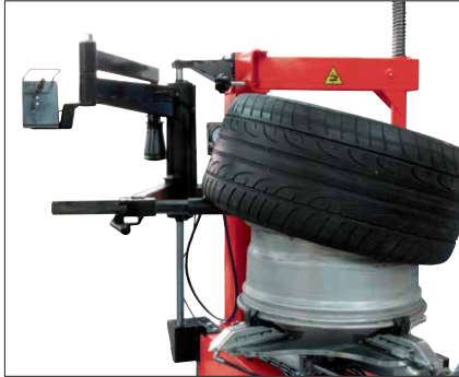
Helper arm demounting lower bead
