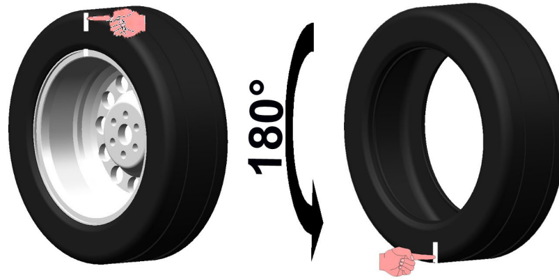
Fig. 81 Position the reference mark on the rim in line with the arrow on the flange
