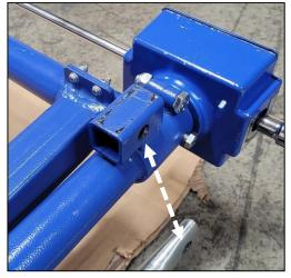
5. Place a Floor Rail on the bottom of lift frame so that the holes for the removed dowel pin are aligned together. Reassemble Floor Rail to lift by inserting longer ±kitqPin, along with Spacer, Washers & Cotter Pins. Ensure Safety Bar & Rail are aligned. Repeat Floor Rail assembly for opposite side.
