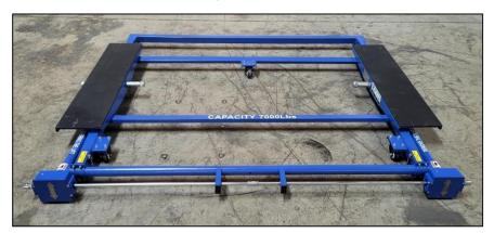
2. Using some form of protection, carefully flip the Lift over onto its topside. Layout Floor Rail parts.
