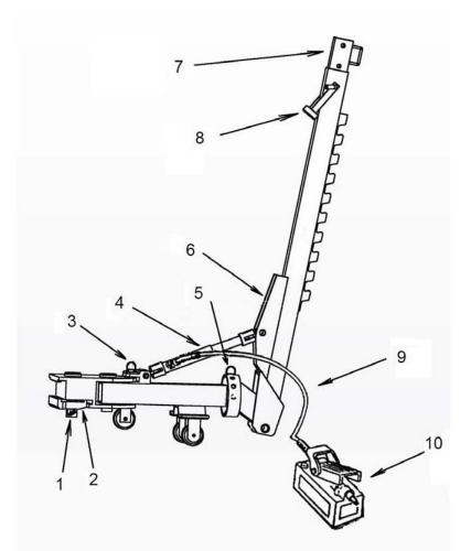
**5.2.2 Specification** Net weight: 1500kg Max hydraulic tension of cylinder: 10t
