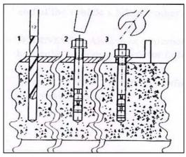
Fig 3.4 The lifting platform must be anchored to the floor
