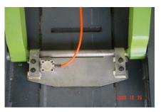
Forbidding: Before that the anti-drop board is in the slot of height limitation, it is forbidden to stretch any part of body under the bench or to start repairing.
