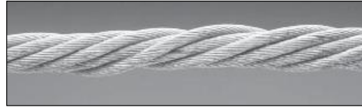
Cable with Necking
